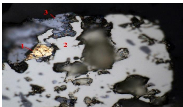
3-rasm. Piritdagi sof oltin Anshilif № 2. Kattalashtirish 100x; analizatorsiz. 1-sof oltin, 2-pirit, 3- galenit.
